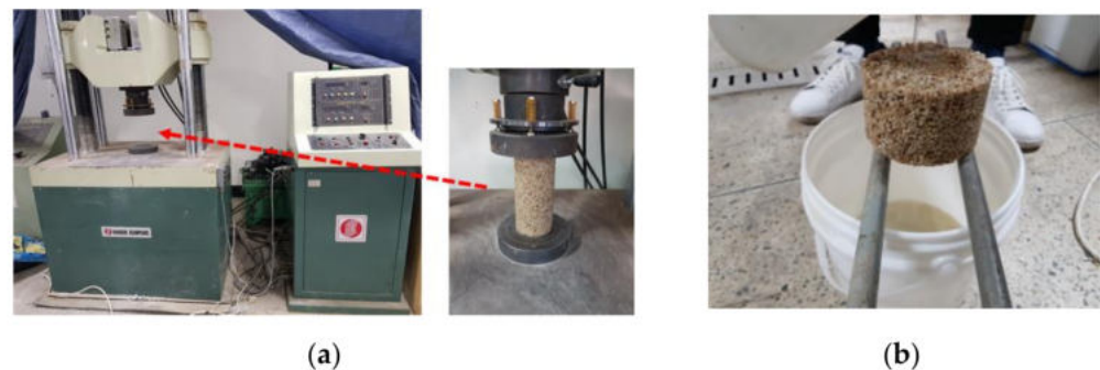
Figure 3. Experimental setup of (a) the compressive strength and (b) the water permeability test.
