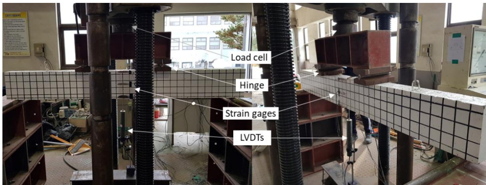
Fig. 5 Test setup of RC beams strengthened with UHPC
